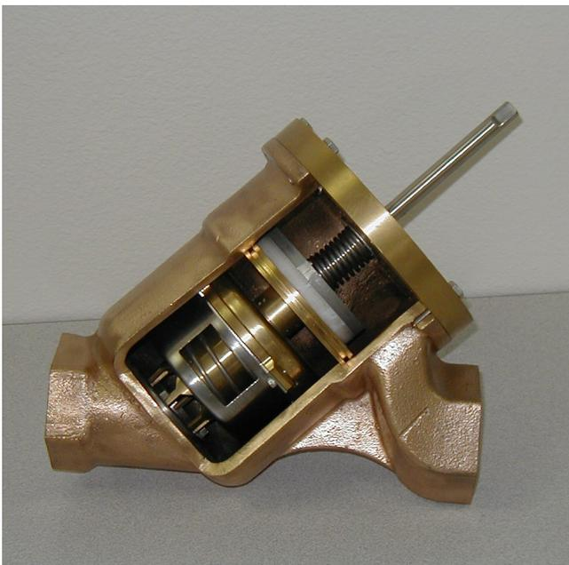
pressure regulator. The piston automatically adjusts such that the pressure drop across the control surface remains constant, even though the pressure difference across the entire valve assembly from inlet to outlet varies. This automatic adjustment enables the control surface to operate independently of system pressure.
